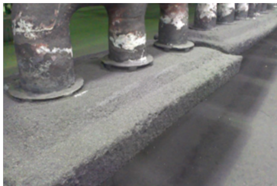
Figure 8. Anode butt with 50 mm “lip”.
