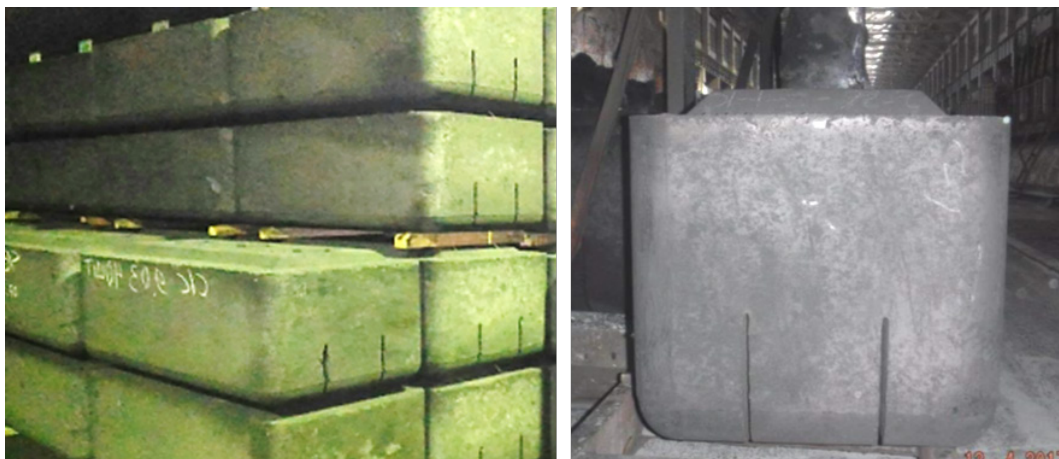
Figure 12. New optimized anode with chamfered edges.
